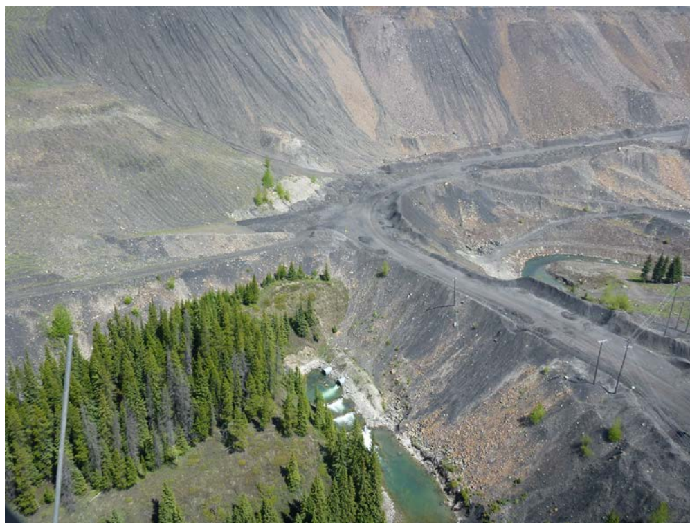
Figure 3.2.14. Henretta Creek Haul Road culvert and the three grouted weir structures illustrating the potential juvenile passage barrier ( i.e. , life stage or partial barrier) approximately 400 m upstream from the Henretta Creek confluence with the upper Fording River.
