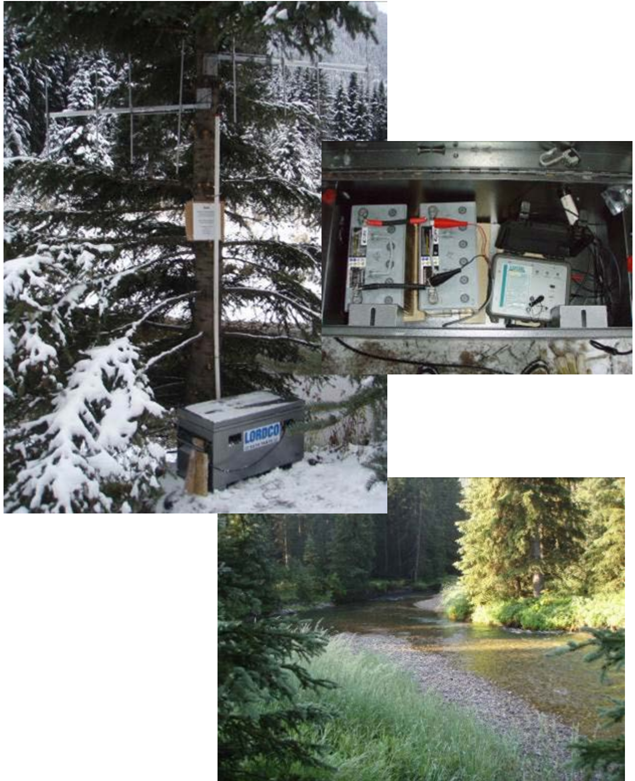
Figure 2.5.1. Photographs illustrating the streamside fixed receiver set-up on a shallow riffle at Station F2 (rkm 48.6); a) antennae and lockbox; b) Lotek SRX DL1 receiver and power source; c) riffle “gateway” habitat selected to maximize detection probability.
