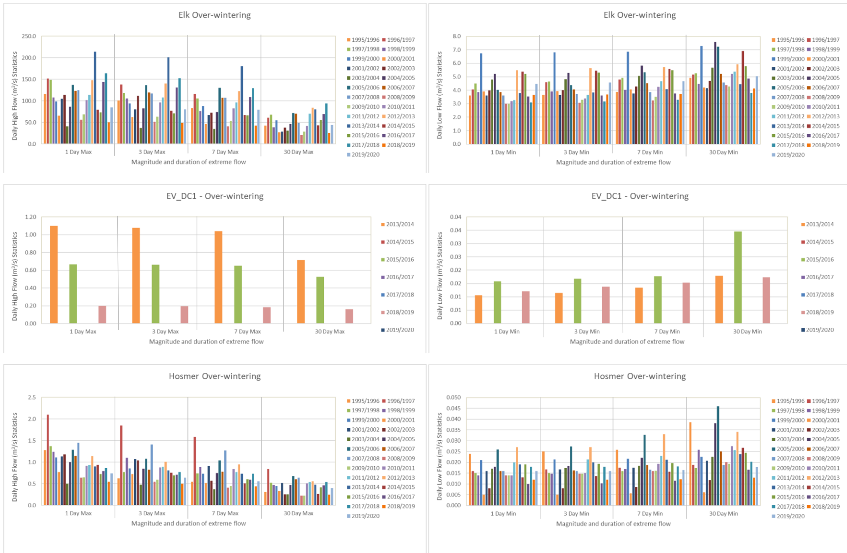
Figure 13. Magnitude and duration of annual extreme streamflow (m 3 /s) at Elk River near Natal, EV_DC1, and Hosmer stations during WCT overwintering (October 11 to May 27). Note the y-axis range is different for each station.
