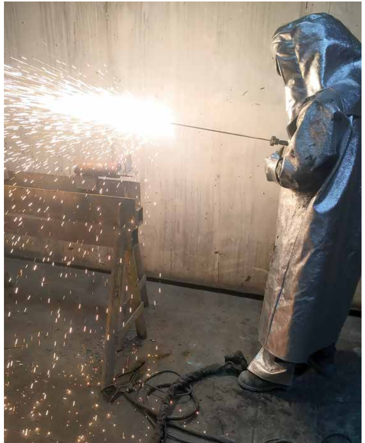
Gabe Schaeffer uses an oxygen lance to pierce steel while at work at Red Dog. Gabe completed his apprenticeship last year as a heavy equipment mechanic.
