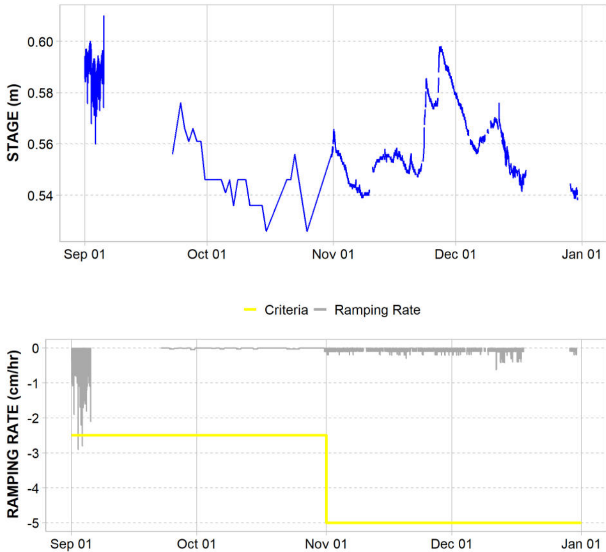
Figure 4. Stage and ramping rate for Measuring Point B during the 2017 period of record. Ramping rate criteria for the fry-present (-2.5 cm/hr) and fry not-present (-5.0 cm/hr) periods are indicated with horizontal yellow lines.
