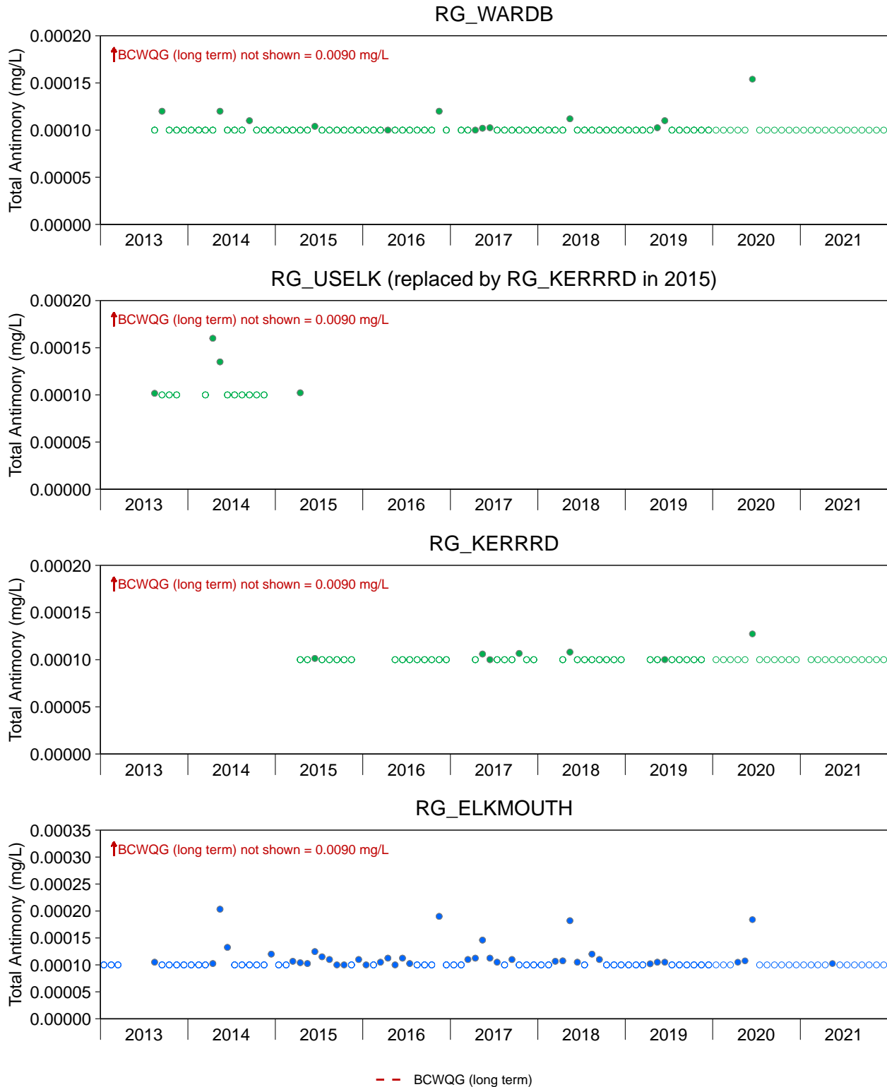
Figure B.1: Monthly Average Concentrations of Total Antimony in the Kocanusa Reservoir Water Quality Sampling Areas, 2013 to 2021
