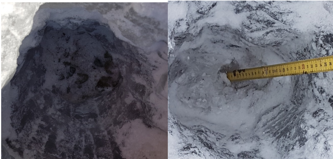
Figure 19. Photo of ice bore hole from FR_FOBCP (left) and FR_FODHE (right) taken on February 11 and 13, 2019, demonstrating freezing of the entire water column.
