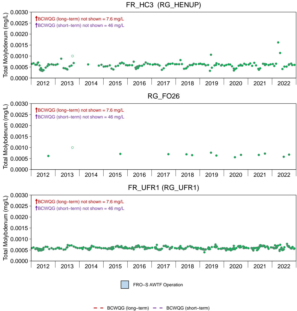
Figure D.11: Time Series Plots for Total Molybdenum Concentrations from FRO LAEMP Sampling Areas, 2012 to 2022
