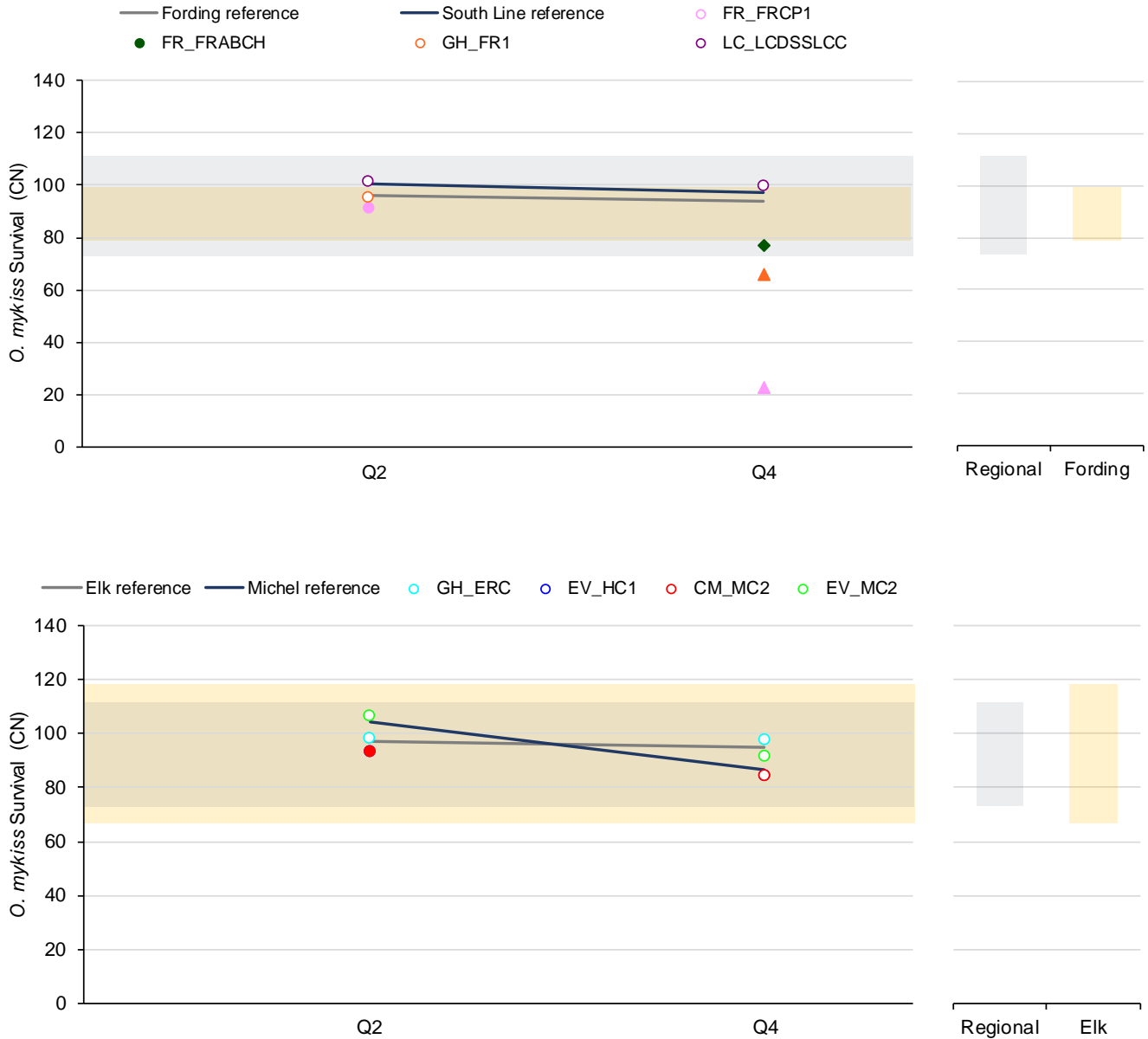
Figure 3.3-15: Mean results for O. mykiss survival in the Fording River reference and its test site waters (top left panel) and the Elk River reference and its paired test site waters (bottom left panel). Regional and local normal ranges (2.5 th to 97.5 th percentile) are shown as bars (right panels).
