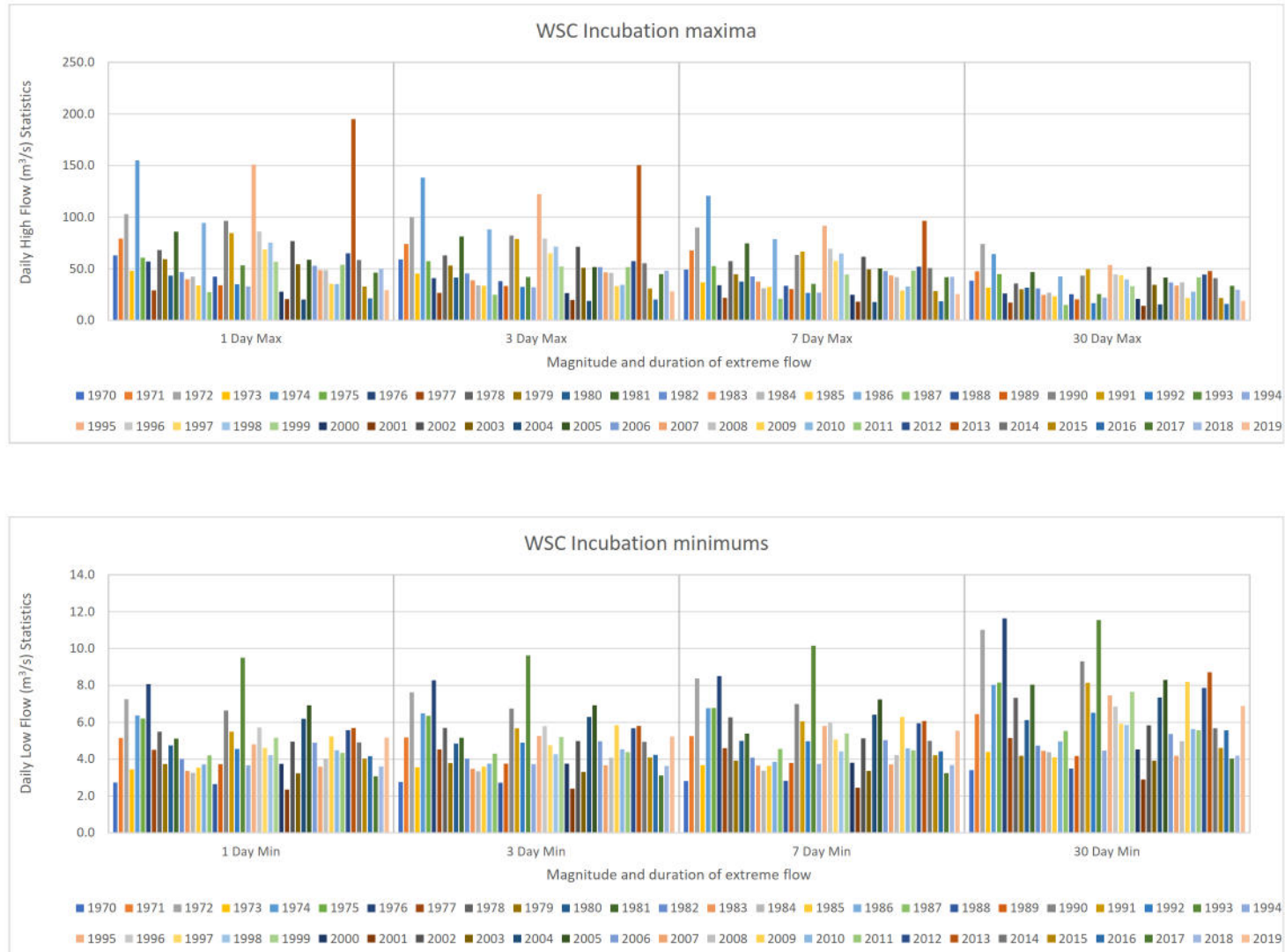
Figure 25. Magnitude and duration of annual extreme streamflow ( m^3/s ) at the WSC Fording River at the Mouth station (08NK018) during WCT incubation (May 15 to August 31). Note the y-axis range is different for each statistic.
