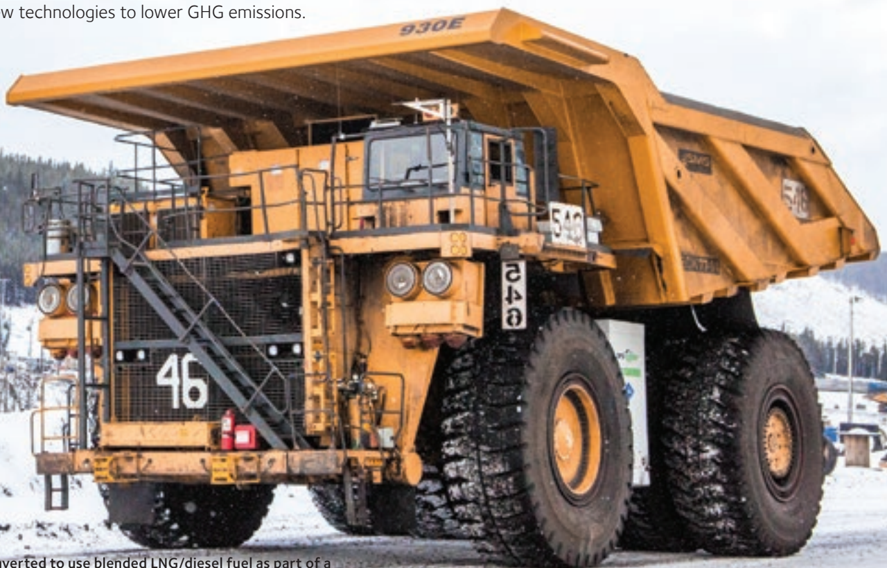
Haul truck converted to use blended LNG/diesel fuel as part of a pilot project at Teck's Fording River Operations.
