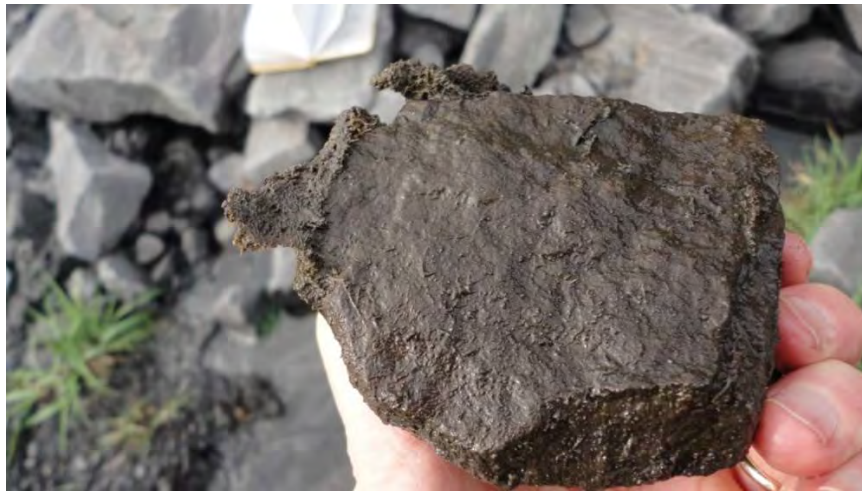
Figure 1. Partially Concreted Sample. Note calcite on the left side edge, which has extended beyond the substrate sample.
