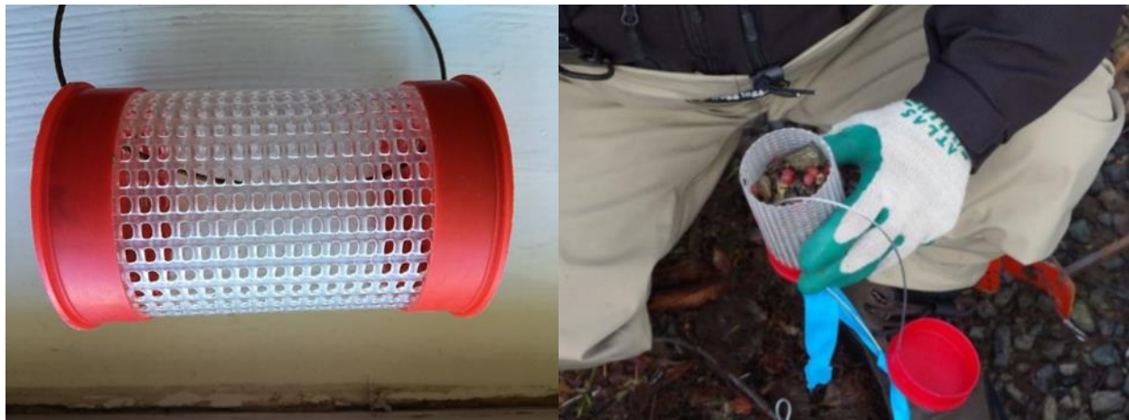
Figure 10. Egg capsule - perforated cylindrical plastic egg tubes (incubators) empty (left) and loaded with substrate (right) consisting of small gravel (2-16 mm diameter).
