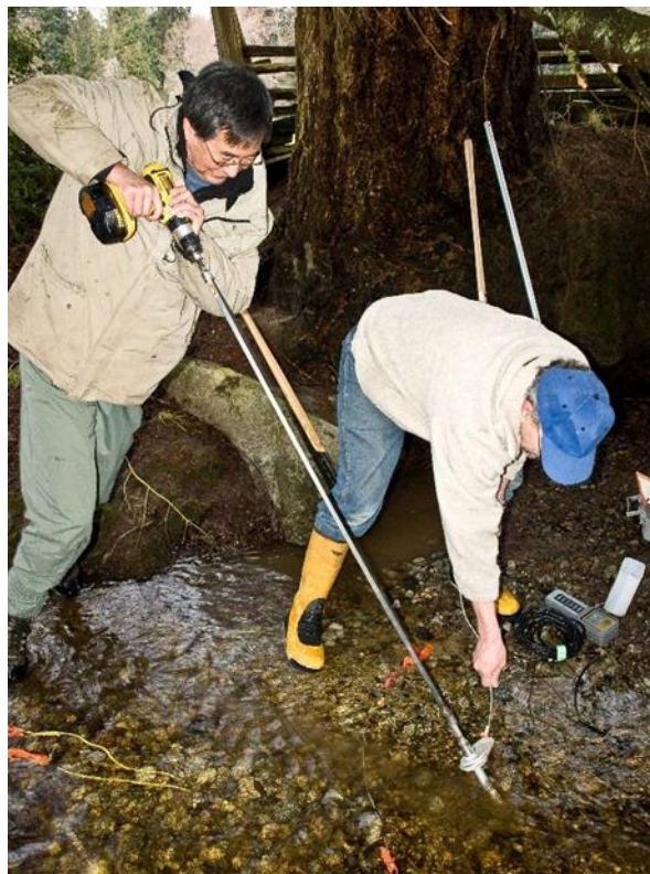
Figure 7. Installation of a pipe incubator using a battery-operated drill.
