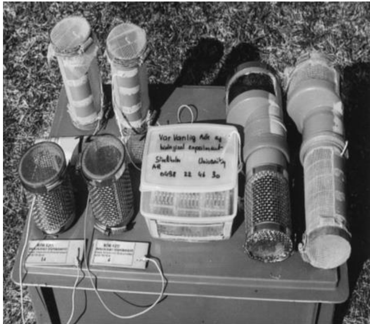
Figure 12. Installation of an egg incubation capsule for salmonids and a diagram of the intragravel fry releaser used at Carnation Creek (top). Also shown are various types of experimental egg incubation capsules (Dumas and Marty 2006) (bottom).
