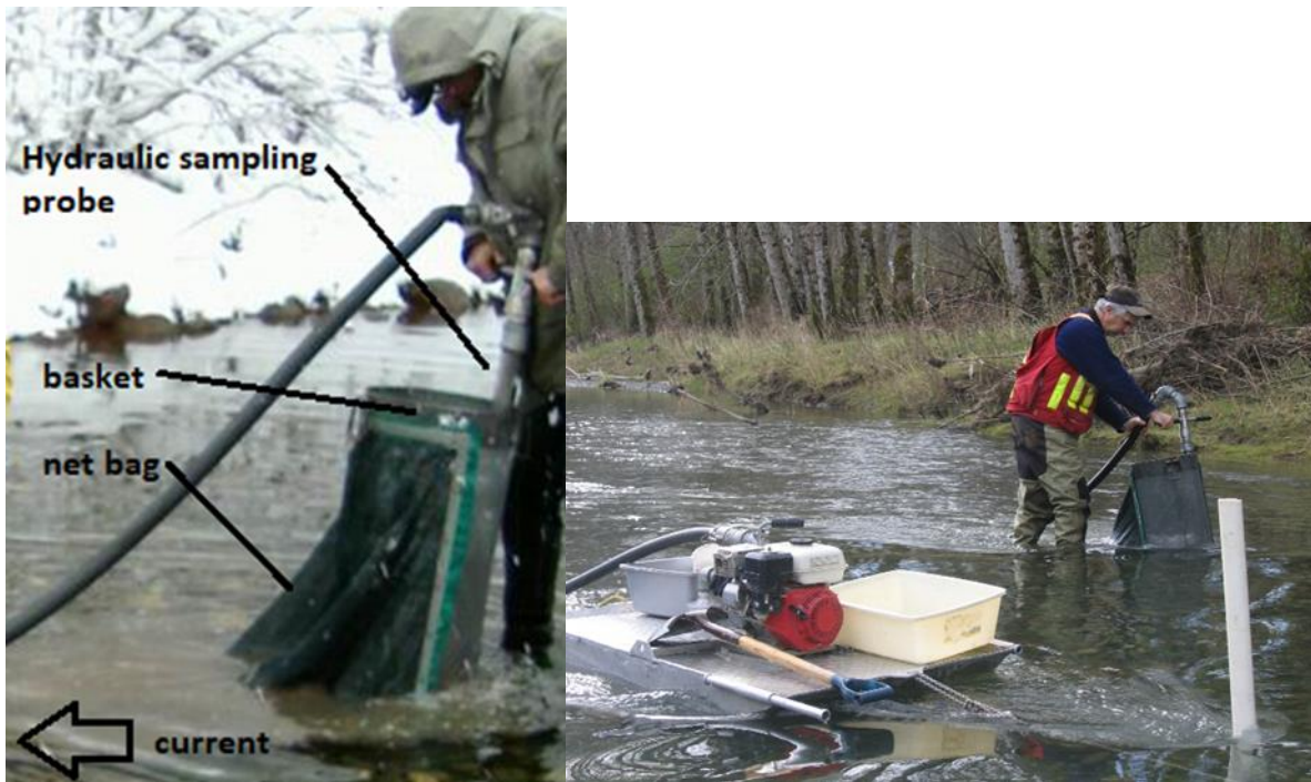
Figure 17. Hydraulic sampling probe, collection basket (left) and water pump on raft (right).
