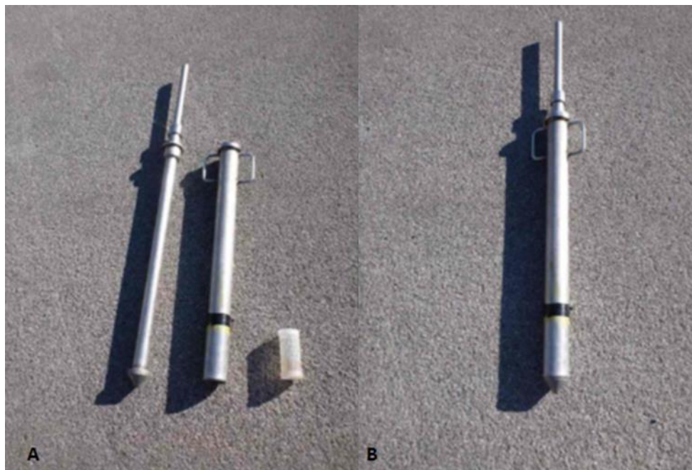
Figure 11. Details of a) egg capsule injection device disassembled with a capsule, b) assembled egg capsule injection device (Dumas and Marty 2006).
