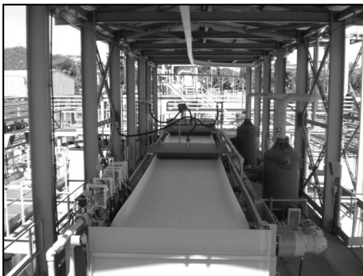
Figure 3: Autoclave Slurry Belt Filter
