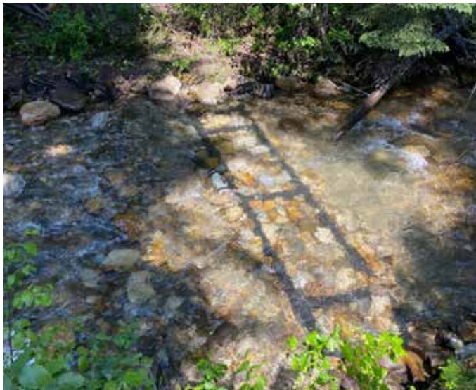
Underwater antenna array used to detect movements of tagged fish in the UFR.
