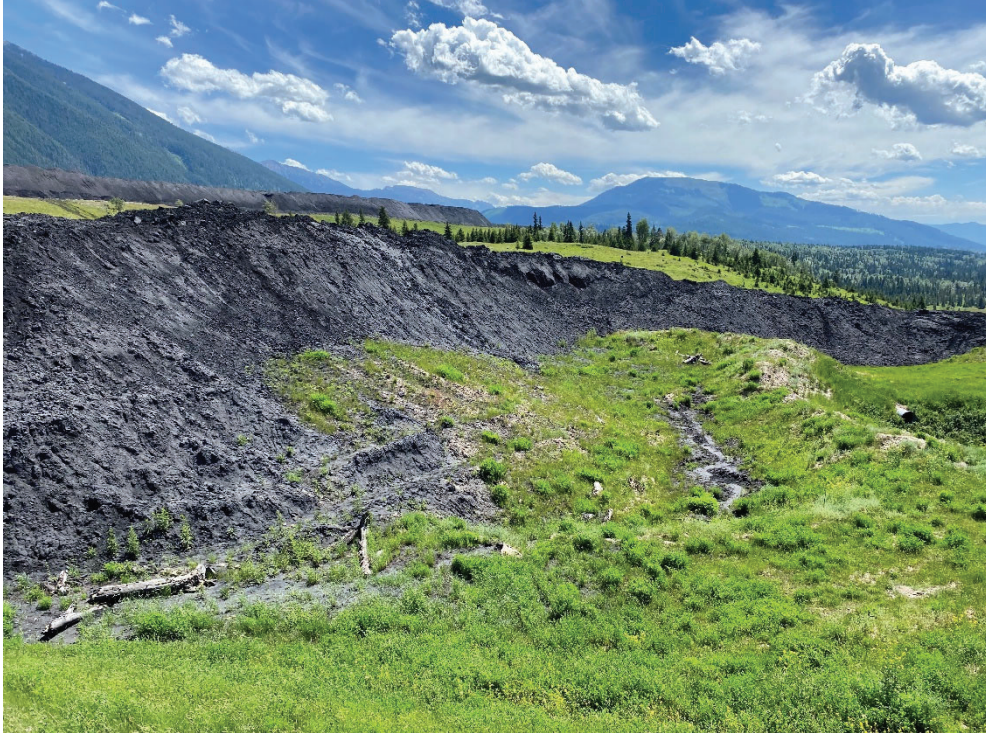
Photo 60. Pond fines deposited on the along the Upper Bench adjacent to the Lower Exfiltration Basin, looking south
