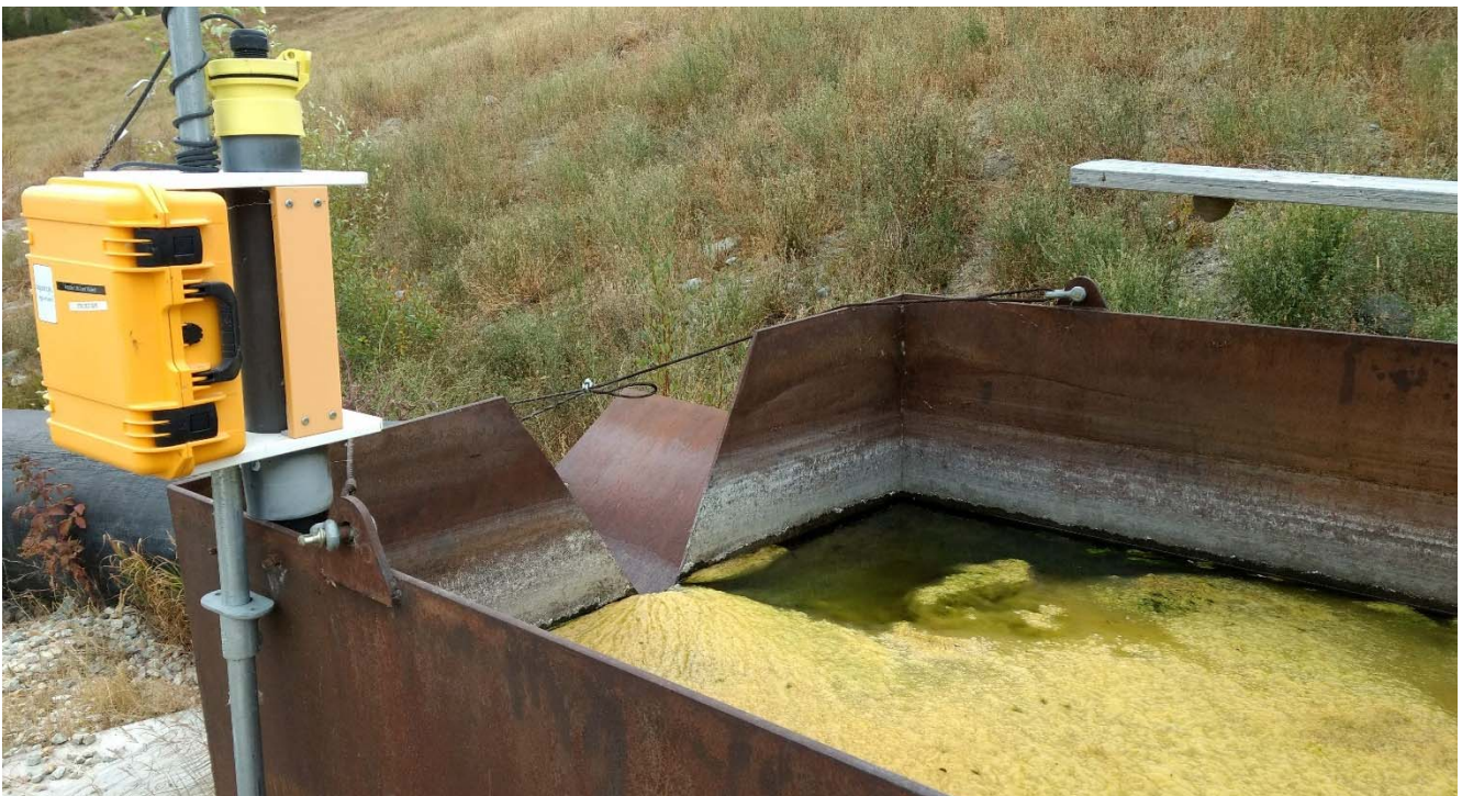
Photo II-B-13 S1: flow measurement weir HM-S1-FS-01 for S1 inflow diverted from Highmont spillway. (HGH-2017-19)
