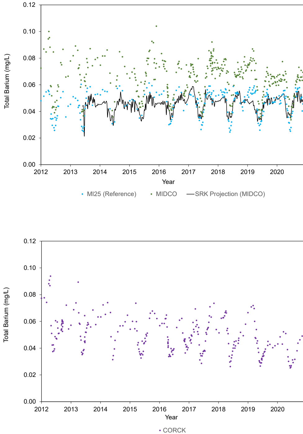
Figure 1.2-4: Temporal Variation in Aqueous Barium Concentrations in Samples Collected from the Coal Mountain Mine Local Aquatic Effects Monitoring Program, 2012 to 2020
