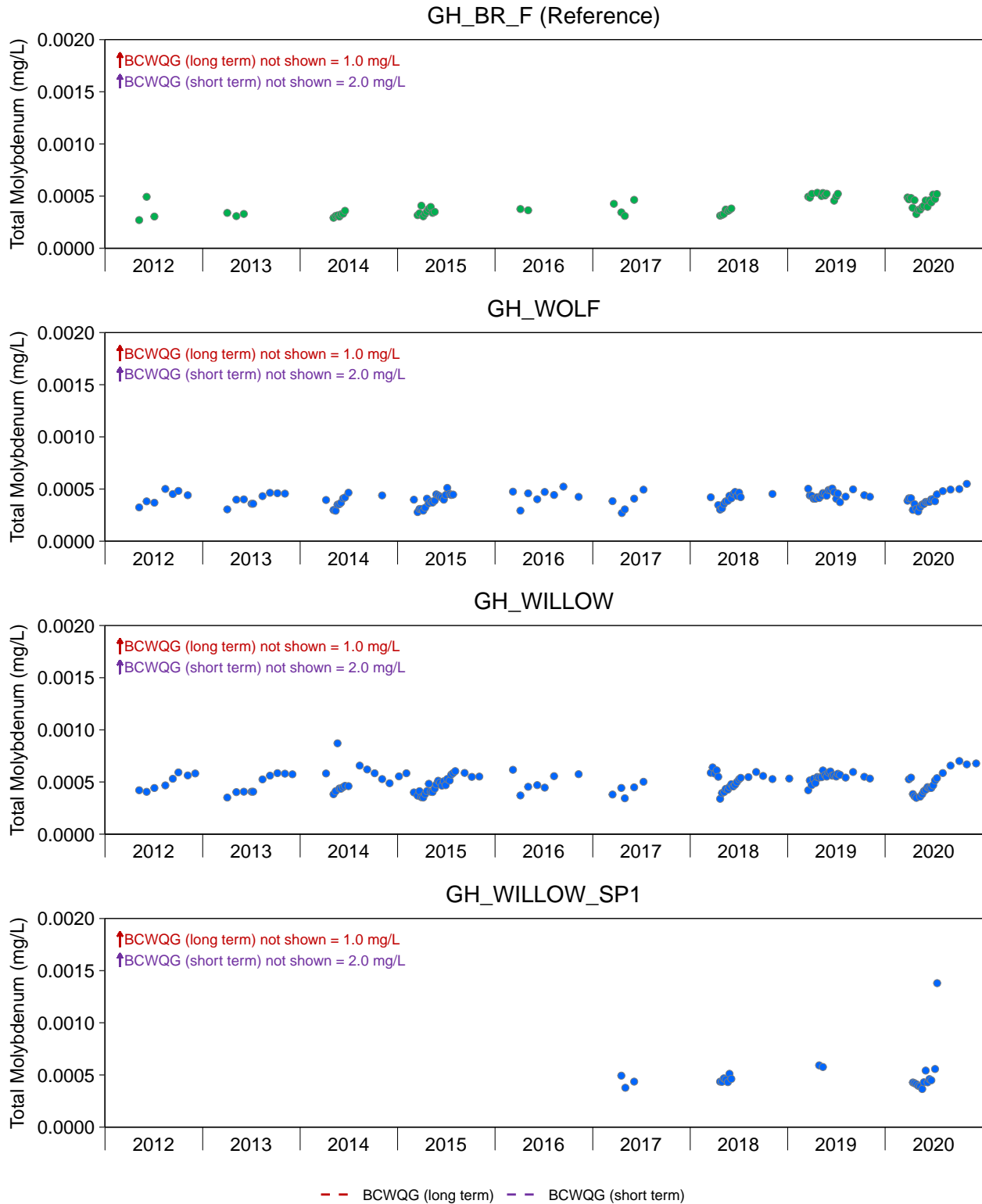
Figure D.15: Concentrations of Total Molybdenum in Samples Collected from the West-Side Tributaries (2012 to 2020) and Monthly Average Rate of Pit Pumping Discharged to Leask Creek and Wolfram Creek (2018 to 2020)
