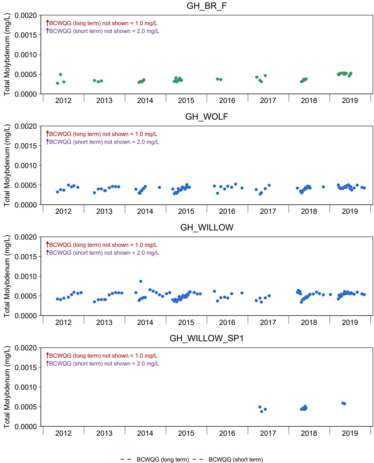
Figure C.8: Time Series Plots for Total Molybdenum Concentrations from the West-side Tributaries, 2012 to 2019
