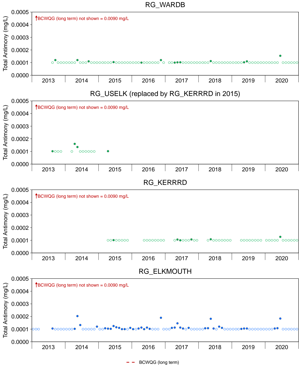
Figure B.1: Monthly Average Concentrations of Total Antimony in the Kocanusa Reservoir Water Quality Sampling Areas, 2013 to 2020
