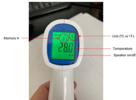
Figure 1 – Thermometer screen (note green screen indicates no high temperature)
