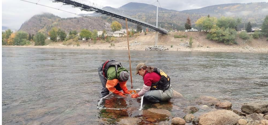
Figure 4: Sampling benthic invertebrates using an area-based approach with a modified surber/CABIN kicknet sampler (devised for area-based sampling in large river system with coarse substrates). The area shown is in Ero-Exp-3 situated on the right bank within the initial dilution zone.
