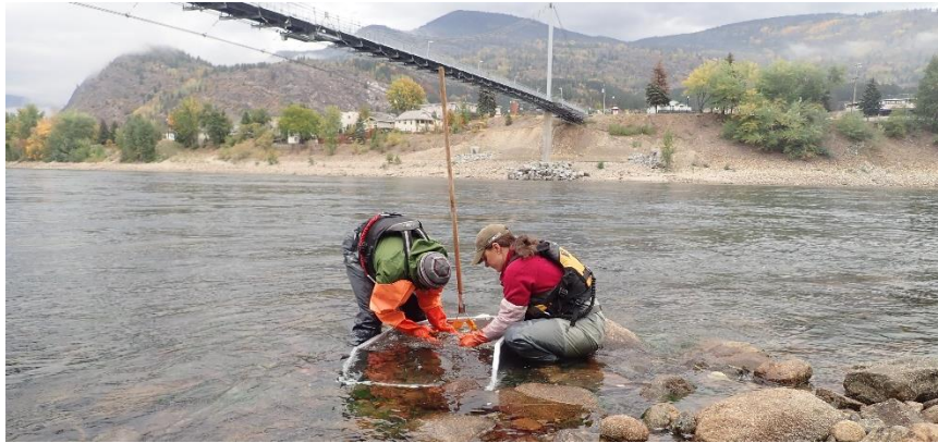
Figure 3-5: Sampling benthic invertebrates using an area-based approach with a modified surber/CABIN kicknet sampler (devised for area-based sampling in large river system with coarse substrates). The area shown is in Ero-Exp-3 situated on the right bank within the initial dilution zone.
