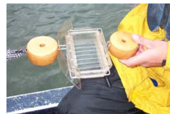
Artificial substrates used to study attached algae
