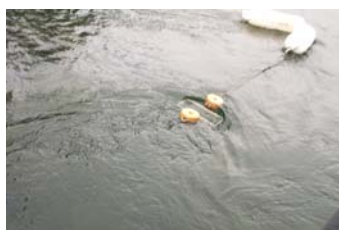
Attached algae sampler in place at the Stoney Creek sampling site
